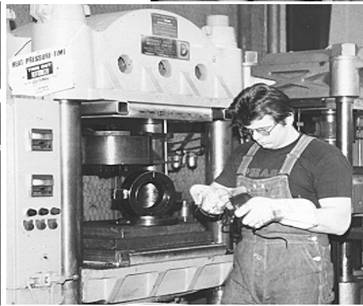
At left spinning of finished part to remove excess flash. Below trimming and final inspection of molded seals prior to packaging and shipment .
