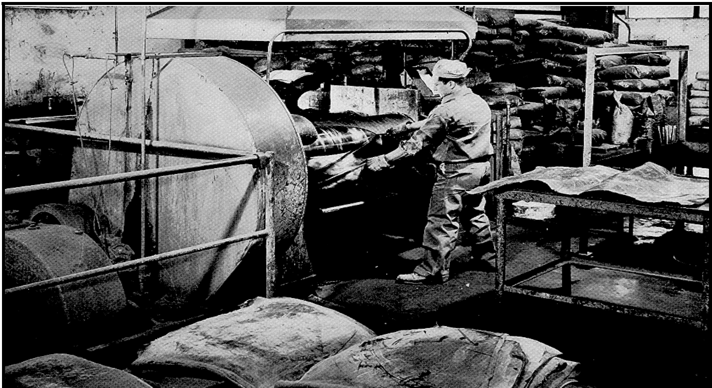
RUBBER MIXING MILL FOR COMMINGLING THE VARIOUS INGREDIENTS IN A RUBBER COMPOUND
